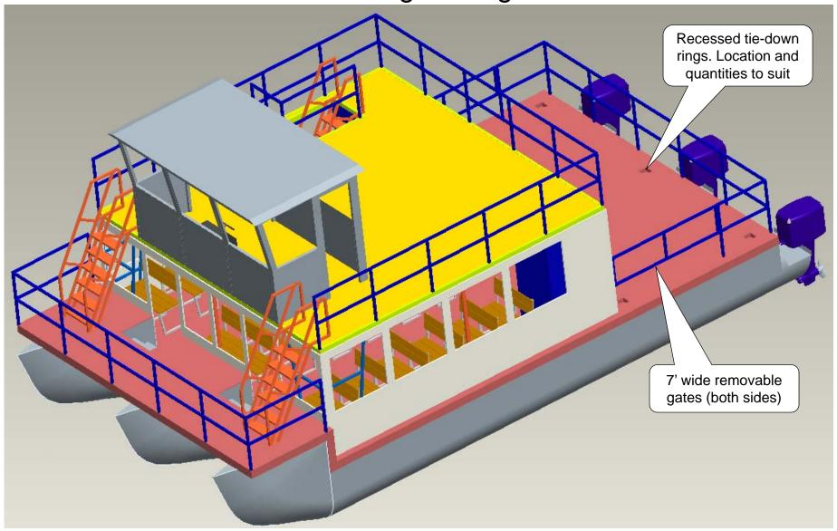
3 x 39" diameter pontoons, double or tripple engine powered 19' x 19' cabin (36-seats, 2-washrooms) with upper deck and 12' x 6' capitain cab 10' x 19' rear cargo deck (7' wide removable gates) and 6'-6" x 20' bow (elevated) deck
